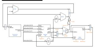
CPI = 1, but long critical path, hardware underutilized. Pipeline:  $f = (\frac{t_{comb}}{k} + t_{setup})^{-1}$ , also latency  $t_{comb} + k \times t_{setup}$  getting worse.
